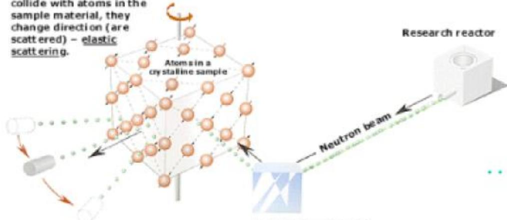
Detectors record the directions of the neutrons and a diffraction pattern is obtained.
